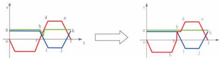
New cam curve and electronic pulsation suppression
